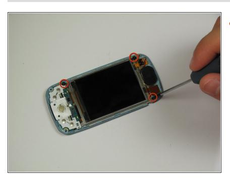
Remove the three 1.75 mm screws.
