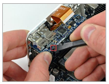
• Use a spudger to depress the small metal finger (shown in red) while lifting the audio board with your thumb.
