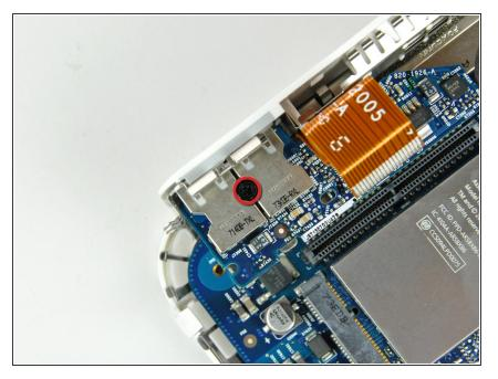
Remove the single Phillips screw securing the audio board to the bottom housing.
