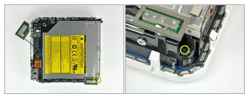
• Remove the Phillips screw from the internal frame near the Bluetooth antenna.
