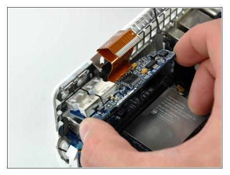
• Lift the free end of the audio board slightly and pull it away from the port side of the bottom housing.
