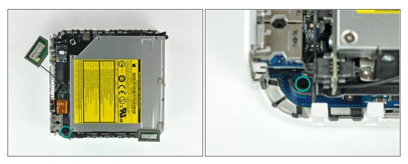
• Remove the Phillips screw near the audio ports securing the internal frame to the bottom case.
