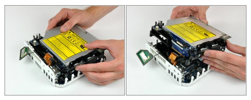
Gently lift the internal frame up from the bottom housing, minding the AirPort antenna and any other cables that may get caught.
