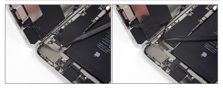
• Use the tip of a spudger or a fingernail to disconnect the front panel sensor assembly connector from its socket.
