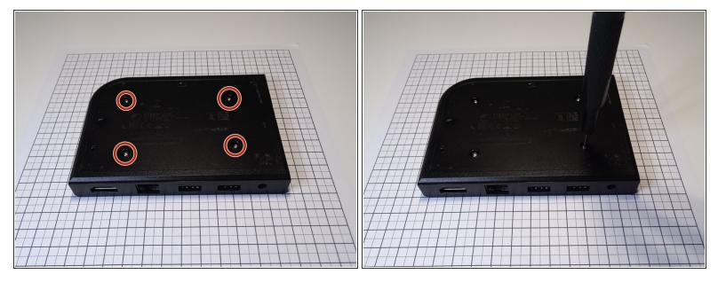
Remove the screws using a Torxx 6 bit
