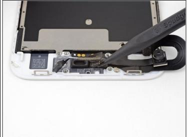
• Slide the tip of a spudger underneath the ambient light sensor flex cable, and lift the sensor out of its housing.
