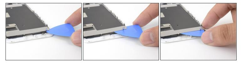
• Insert an opening pick from the bottom right corner and continue to separate the display cable from the LCD shield plate.
