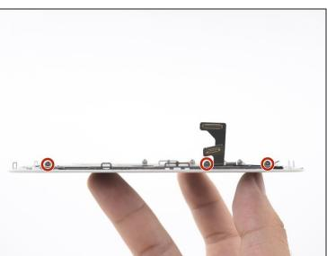
• Remove the three 1.2 mm Y000 screws from either side of the display for a total of six screws.
