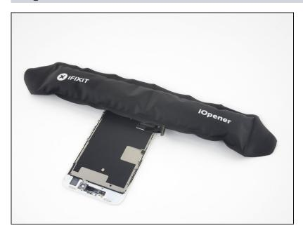
Heat an iOpener and lay it over the edge of the shield closest to the home button to soften the adhesive holding it in place.
