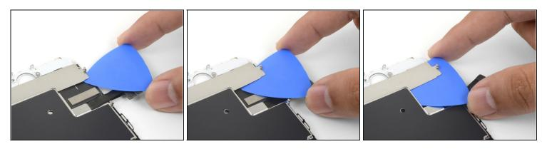
• Use an opening pick to break up the adhesive near the home button that holds the flat display cable to the LCD shield plate.
