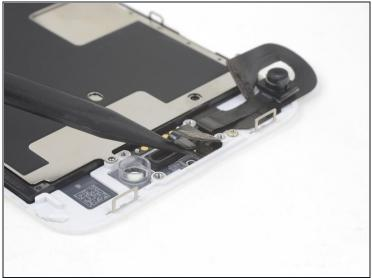
• Use the point of a spudger to gently pry the proximity sensor out of its recess on the front panel.
