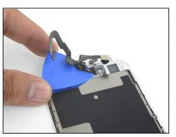
Slide an opening pick underneath front camera cable assembly, separating the adhesive holding the camera and sensor cable.
