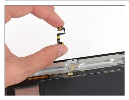
• Remove the microphone from the rear case of the iPad.
