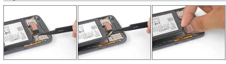
• Using a pair of tweezers or your fingers, grab the black battery pull tab and slowly pull it upwards until the corner is loose.
