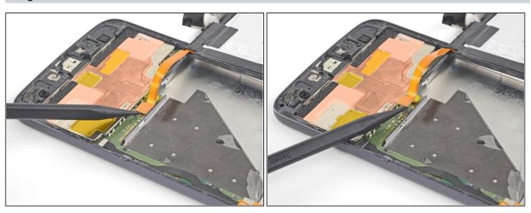
• Using the point of a spudger, pry up the battery connector from its socket.
