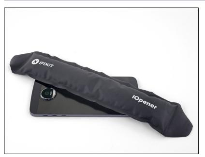
Lay a <u>heated iOpener</u> on the back of the phone as shown for as least 90 seconds.
