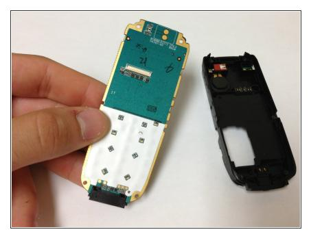
After removing the screen, you will find the charging port located at the bottom of the phone.
