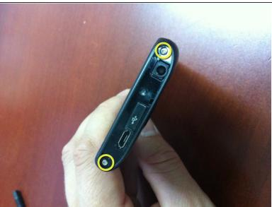
There are six screws to remove from the rear of the phone and two from the top.
