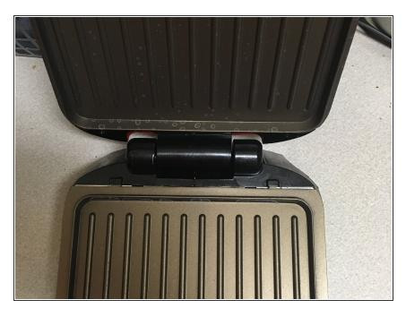
• Open the appliance by lifting the top plate away from you.
