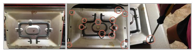
(i) Underneath where the plates sit you will see a coil and 12 screws holding the base plate in place.
