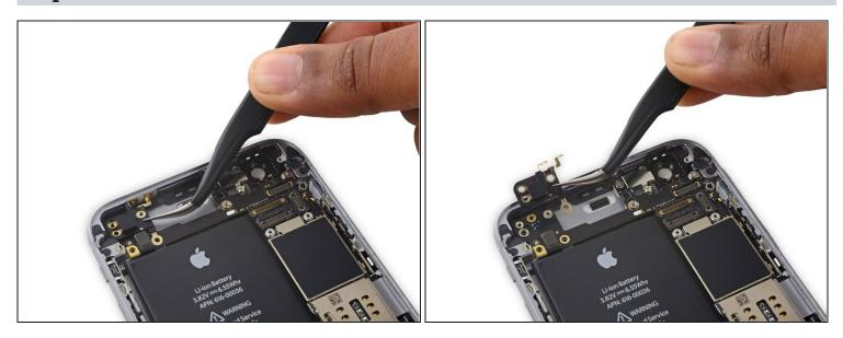
• Remove the top left Wi-Fi antenna.
