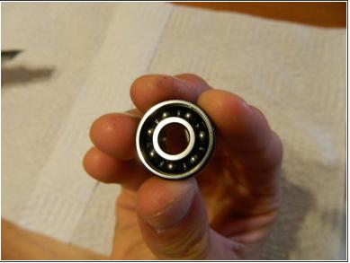
Remove ONE shield from your bearing using the small point of a utility knife. This will allow the chemicals to enter the bearing more freely when the bearing is submerged.
