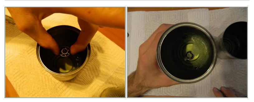
Submerge your bearing in the cleaning container for 15 - 20 seconds to allow the solvent to soak into the bearing.
