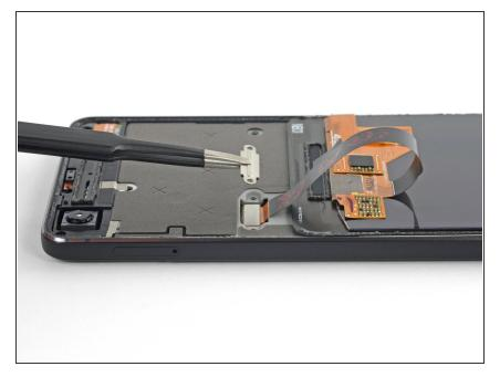
• Remove the display cable bracket.
