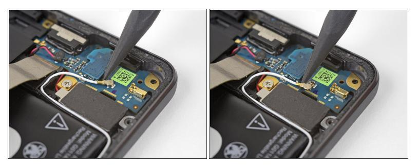
Use the point of a spudger to pry the white antenna cable connector straight up and disconnect it from the charging assembly board.
