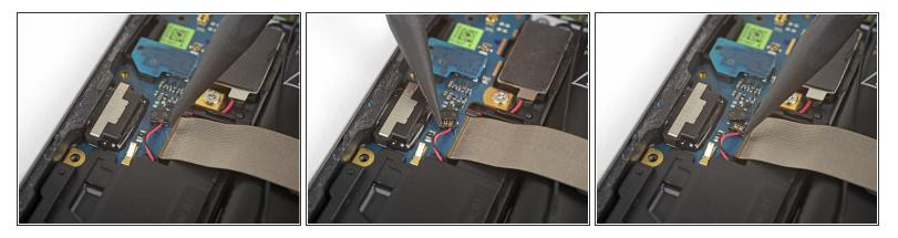
• Use the tip of a spudger to gently push the speaker cable connector out of its socket horizontally, alternating pushing either side of the connector out a little bit at a time.
