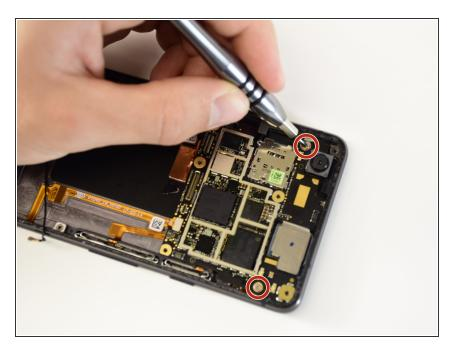
Remove the two 2.5 mm PH00 screws.
