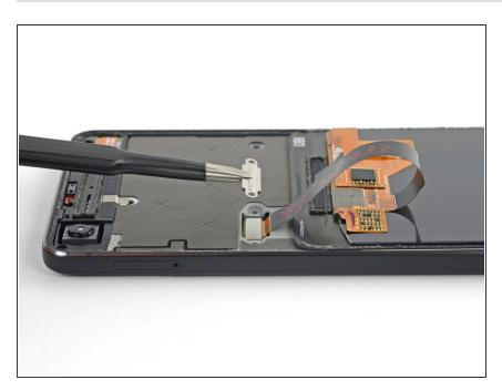
• Remove the display cable bracket.
