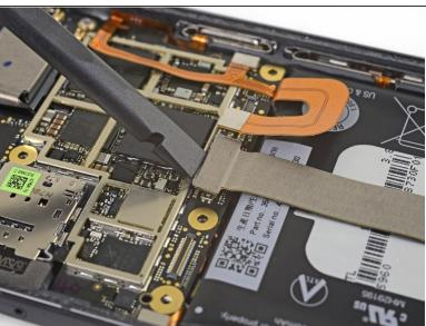
use the flat end of a spudger to disconnect the charging assembly connector from the motherboard.
