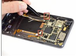
• Disconnect two connectors at the bottom edge of the motherboard.
