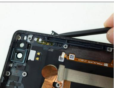
Push the external power and volume buttons out of the case with a spudger.
