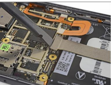
Use the flat end of a spudger to disconnect the charging assembly connector.
