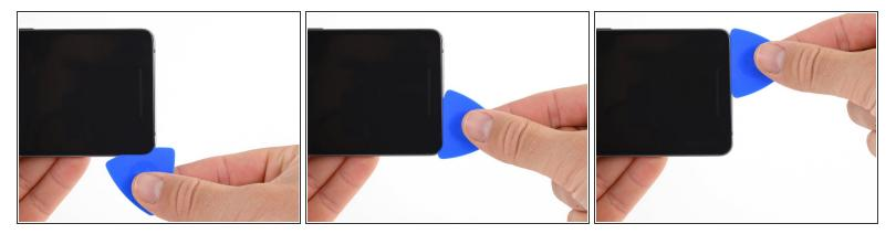
Slide the pick around the bottom-left corner and along the bottom of the phone. Keep pick at a slight angle away from the screen to avoid damage to the OLED corners.
