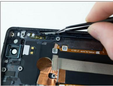
Remove the remaining button halves with a pair of tweezers.
