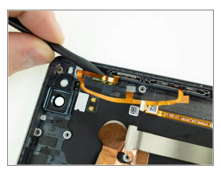
Use the pointed end of a spudger to gently lift up the button ribbon cable from the phone.
