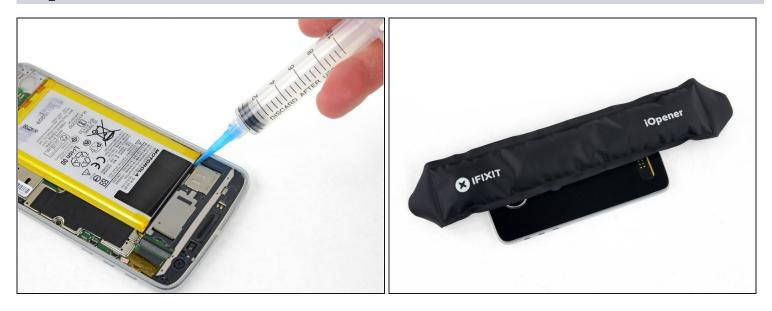
(i) The battery is strongly glued into place.
