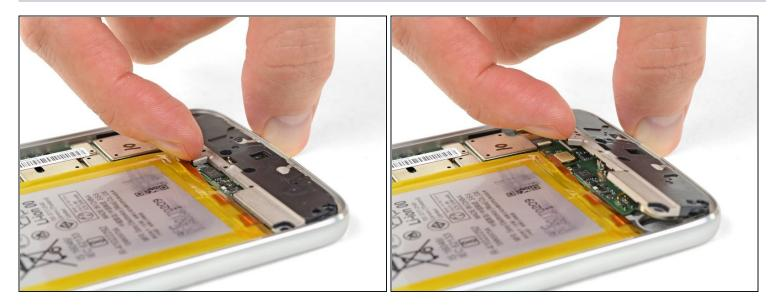
Pry up and remove the lower cover.
