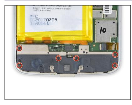
• Use a T3 Torx driver to remove the six 3.2 mm screws securing the lower cover.
