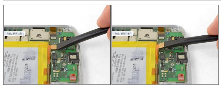
• Use a spudger to disconnect the battery by prying its connector straight up from the motherboard.
