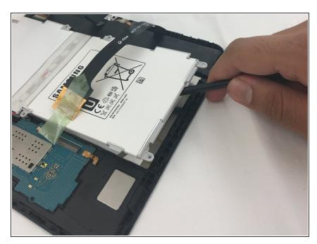
Use the nylon spudger to remove the battery by prying up on the edges.
