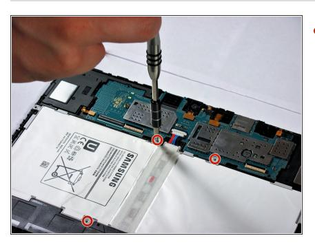
Use a Phillips #00 screwdriver to remove the four 3.2mm screws.
