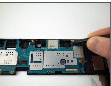
Pry up and disconnect the power and volume button press-fit connector with the flat end of a spudger.
