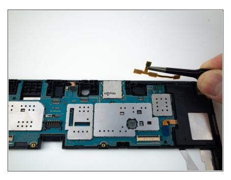
Remove the power and volume button ribbon cable.
