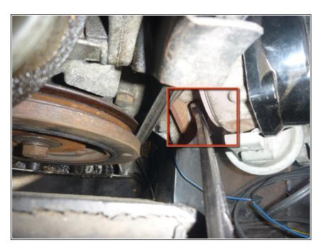
Using a 9/16 inch wrench, loosen the distributor adjustment bolt and leave the wrench in place
