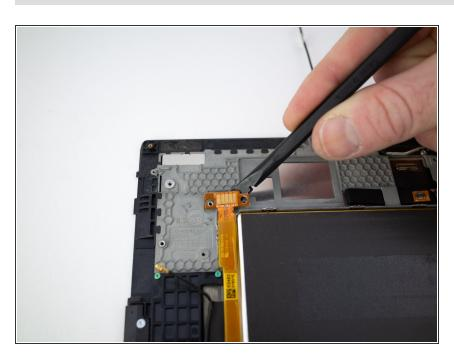
Pry up the battery connector with the flat end of a spudger.
