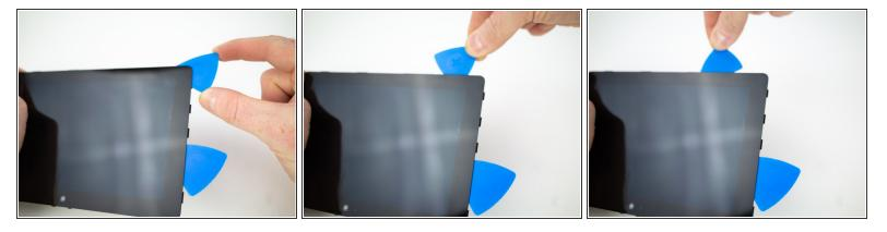
Roll the second opening pick all the way around the perimeter of the display.
