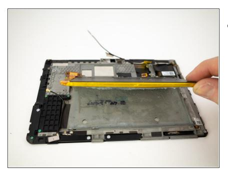
Remove the battery from the midframe.
