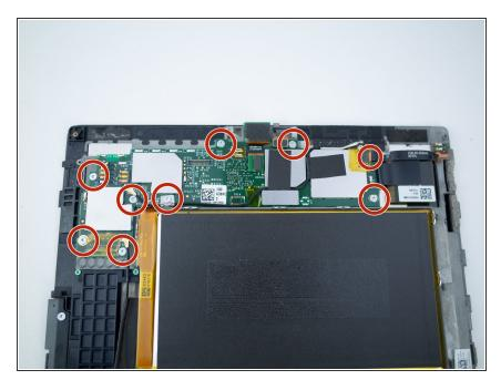
Remove the nine 3mm T6 Torx screws from the motherboard.
