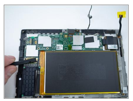
Use a spudger to disconnect the second antenna cable from the motherboard.
