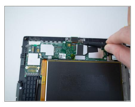
Use the flat end of a spudger to disconnect the front camera press-fit connector from the motherboard.
