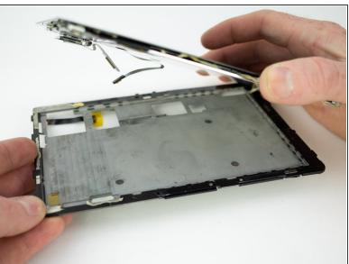
• Lift up on the glass display to remove it from the metal mid-frame.
