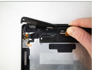
Pry up the left speaker with the flat end of a spudger and remove.
