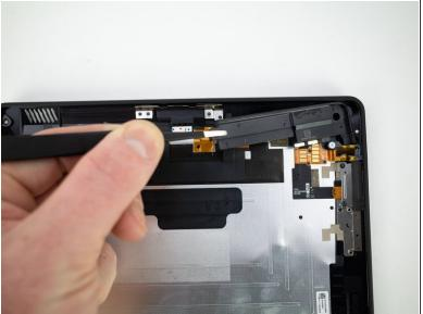
Pry up the right speaker with the flat end of a spudger and remove.
