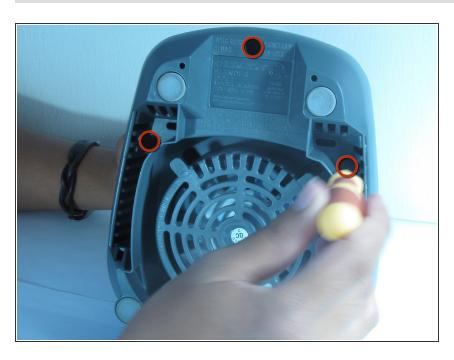
Remove the top three 1/4 inch base screws using a Philip's head screwdriver.
