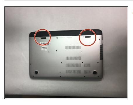
Flip over your HP Pavilion to the backside, so you see the battery release and battery unlock slide mechanisms.
