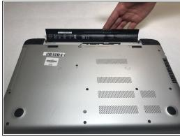
• On the right side of the laptop you will see the slide release mechanism and slide it to the left, then the battery will pop out.
