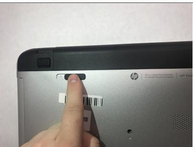
On the left side on the back of the laptop, you will put your thumb on the unlock slide mechanism and slide it to the right.
