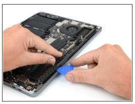
Use an opening pick to lever out the antenna cable assembly in the areas shown.
