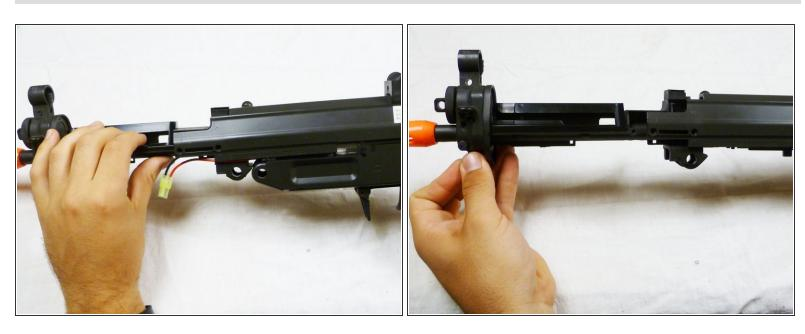
Carefully tug on the tip of the gun and pull the barrel and its cover out.
