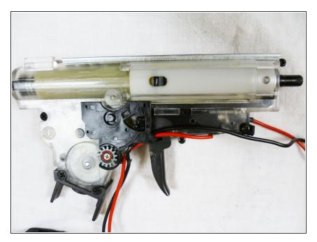
Using a Phillips #0 screwdriver, remove the single 3mm screw holding the safety/trigger cover in place.
