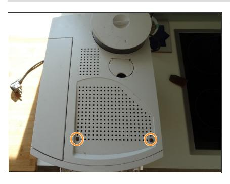
Remove the two Torx T10 screws on the top.
