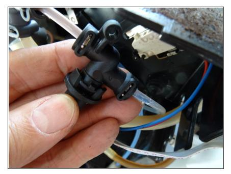
Look for the outlet valve on the top right of the device.
