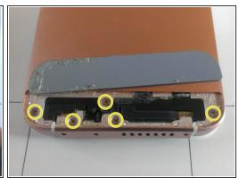
To remove the bottom cover, pull it upward.
