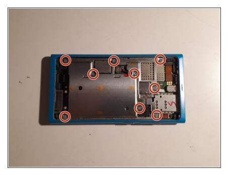
Unscrew the marked screws using the T4 torx screwdriver.
