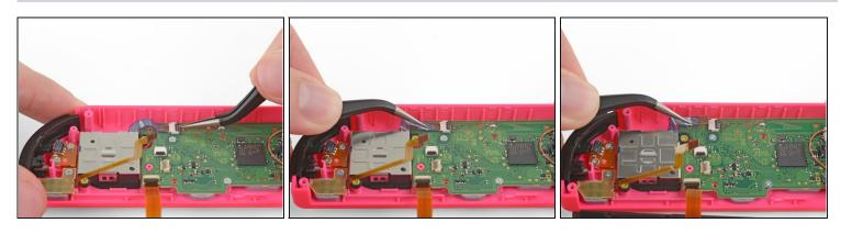
• Finally, the joystick is locked into place by one last ZIF connector. Carefully flip the ZIF lock upward and disconnect the cable.
