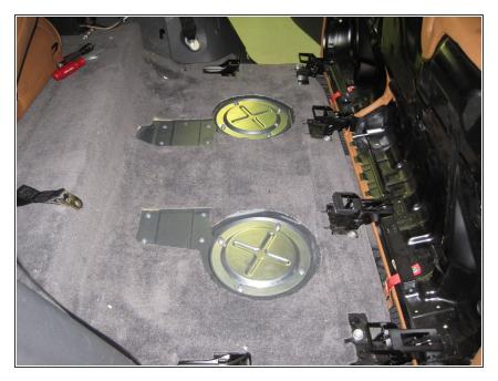
• Install the covers back on top of the gas tank ports.
