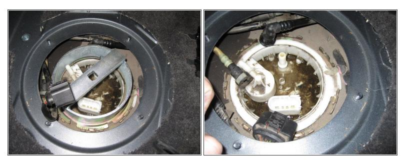
• Use the T10202 tool again here to remove the retaining ring. Set the ring aside.
