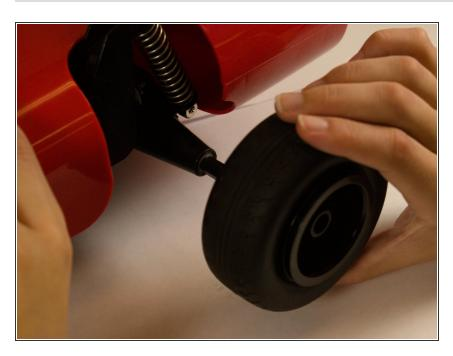
After removing the 11 mm screw, firmly grip the wheel and pull away from the vehicle.
