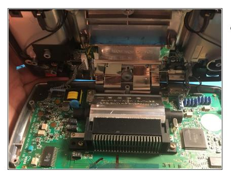
Carefully lift up the back half of the case. There are cables connected to the back case that will need to be unplugged before the back can be fully removed.
