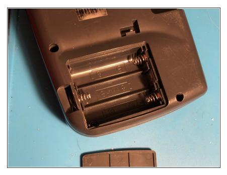
Pop open the two battery compartment covers on the back of your Game Gear and remove the batteries.
