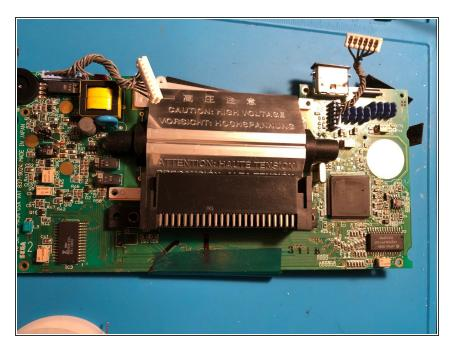
Remove 8 Phillips screws and lift the main circuit board out of the case.
