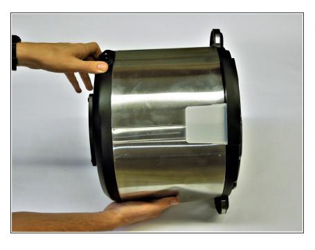
Reorient the crockpot on its side to prepare for the heating element removal.
