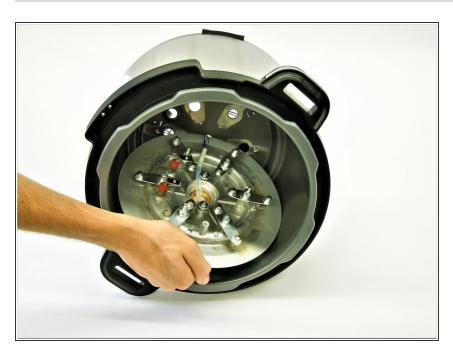
Carefully pull the heating element out and rotate it until bottom side is facing up out of the pot.
