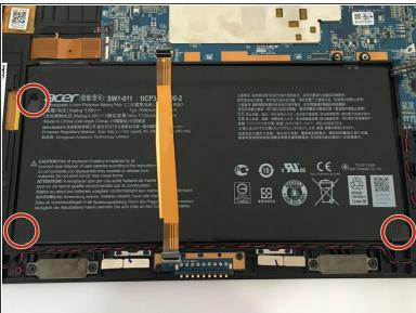
Peel back the black tape holding the battery in the three corners of the battery.
