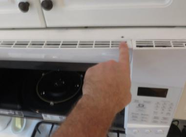
The first step is to remove the two philips screws located on the top of the microwave. These two screws hold the exhaust fan cover.
