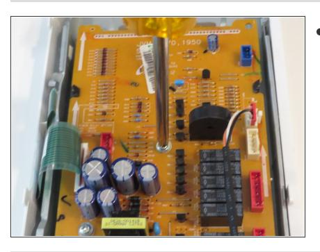
The circuit board is held on with 3 phillips screws, shown here, plus a metal band.
