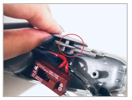
Remove the settings switch by lifting straight up.
