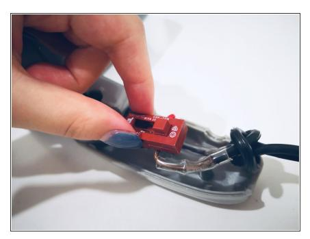
• Remove the internal switch from the rear portion of the handle.
