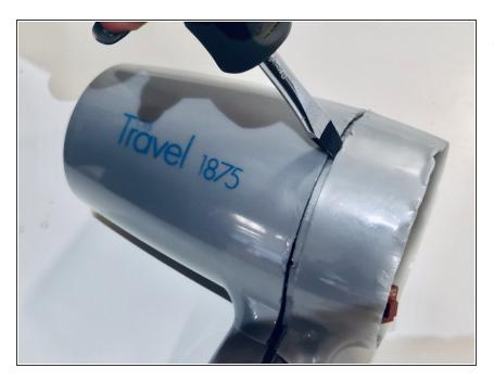
Separate the back and front case by using the 6.5mm flathead screwdriver.
