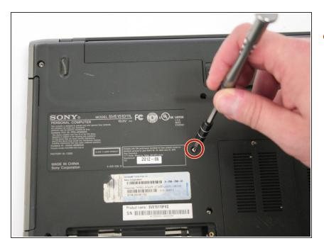
Use a Phillips #0 screwdriver to remove the one 4.0 mm screw next to the model number label.
