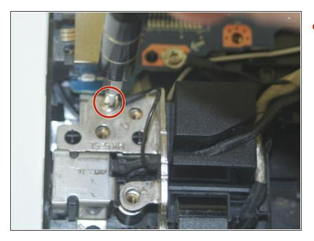
Use a Phillips #0 screwdriver to remove the one 3.0 mm screw attaching the grounding wire to the left lid hinge.
