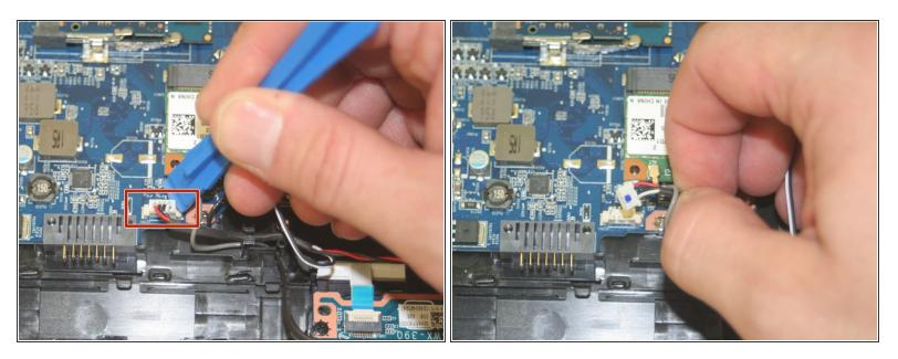
• Use a plastic opening tool to unsecure the white speaker wire connector on the motherboard.
