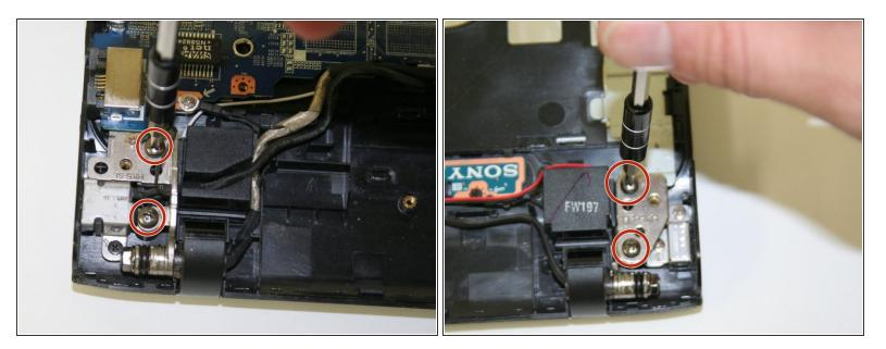
Use a Phillips #0 screwdriver to remove the two 9.0 mm lid hinge screws next to the left and right speaker unit.
