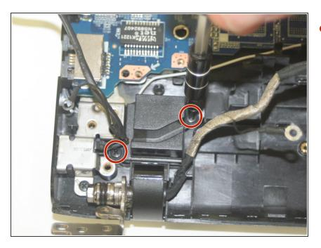
Use a Phillips #0 screwdriver to remove the two 3.0 mm screws securing the left and right speaker unit to the laptop.
