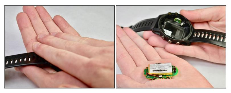
• Lift the watch and turn it over one hand. The motherboard should fall out easily.
