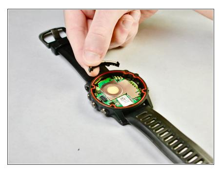
• Carefully remove the antenna, and set it aside.
