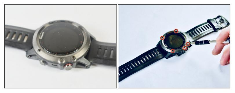
• Use a T6 screwdriver to remove the five 1.7 mm screws from the watch face.
