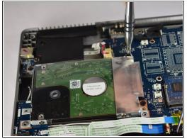
Unscrew the four 4mm PH0 screws holding the hard drive in place.
