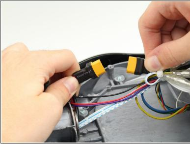
Disconnect the circuit boards from the battery by pulling both battery connectors apart.
