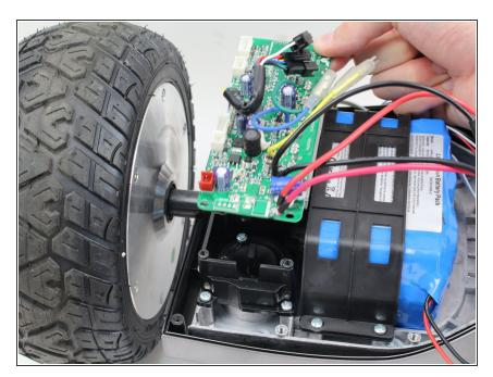
Remove the circuit board by pulling it up and out of the hoverboard.
