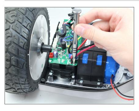
Remove the four 14mm Phillips #1 screws in the corners of each circuit board by turning the screwdriver counterclockwise.
