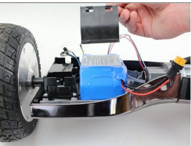
Lift the battery cage up and off the battery.
