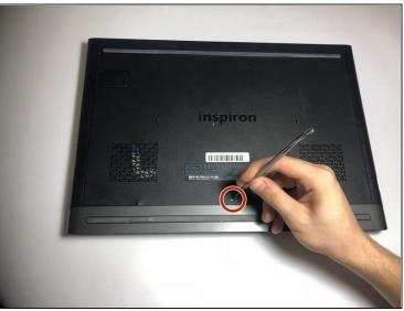
• Remove the 3mm screw in the location shown, using a Phillips #1 screwdriver.
