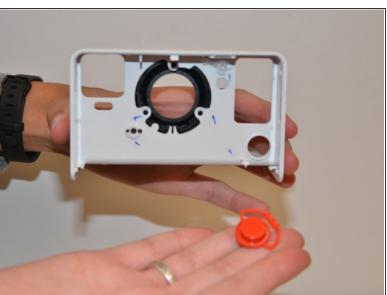
With force pull the shutter button away from the white piece of the camera.
