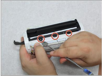
• Use the spudger to reach under the sides of the black centerpiece to access the six latches, three of which are on each side.
