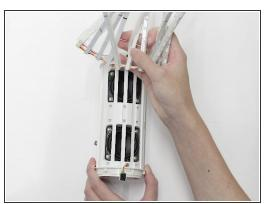
Manually remove the LED strips from the outside of the white plastic casing.
