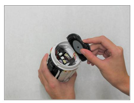
Remove the other end of the device to access the wiring underneath it.
