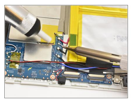
Desolder the battery connectors from the motherboard.
