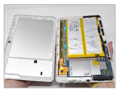
Separate the back panel from the rest of the device.
