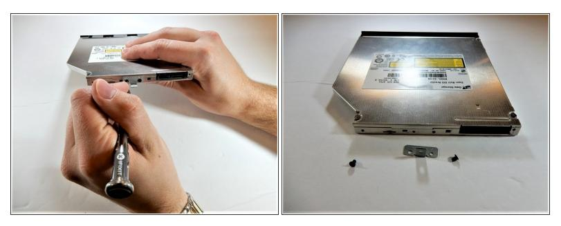
• If needed, the small plate can be removed by unscrewing the two .4 centimeter Phillips screws.
