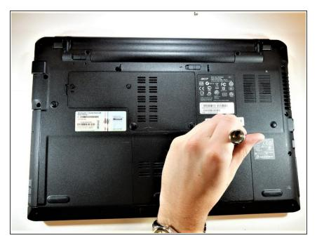
Unscrew the two .8 centimeter screws on the bottom plate with the PH #0 screwdriver.
