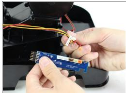
Pull the daughterboard out of the device and remove the three-prong connectors by using your hands.
