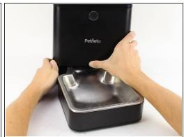
• Eject the SmartBowl by pressing the button located at the front of the SmartFeeder base.
