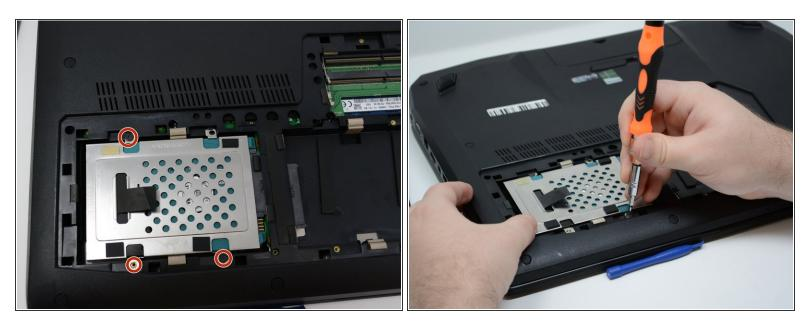
• Remove the three 4mm Phillips #2 screws.
