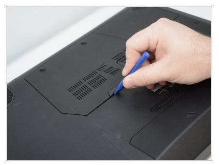
With the computer upside down, lift up on the rubber cap on the back plate to access the captive Phillips #2 screw.
