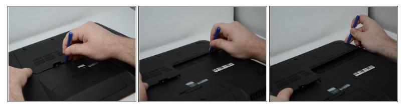
• Pry around the edges of the plate using a plastic opening tool until the plate is removed.
