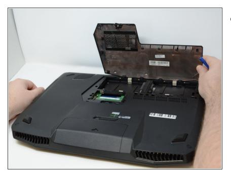
• To access the hard drive, remove the back plate.
