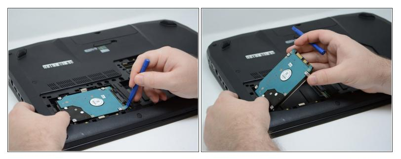
• With the hard drive exposed, pull the hard drive away from the connection point and then remove the hard drive.
