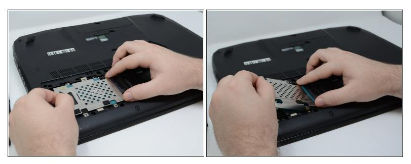
Pull back on the tab on the hard drive shield until it is clear of the screw slots. Next pull the shield out.
