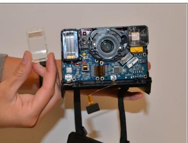
Forcefully pull on the flash cover until it is removed.
