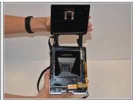
Unscrew the four 5mm screws on the base of the camera. Remove the two pieces of the base.
