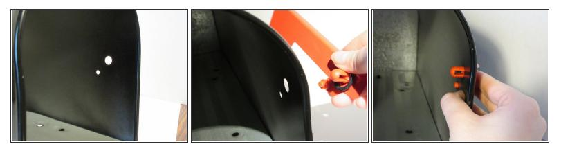
Insert the bracket of the assembled flag through the holes on the outside of the mailbox.
