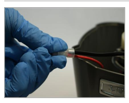
Pinch perpendicular to the flat surface and pull out the black wire.
