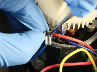
Remove the 2 black, yellow, and red wires from circuit board by push down on the tab to release and then pull up.
