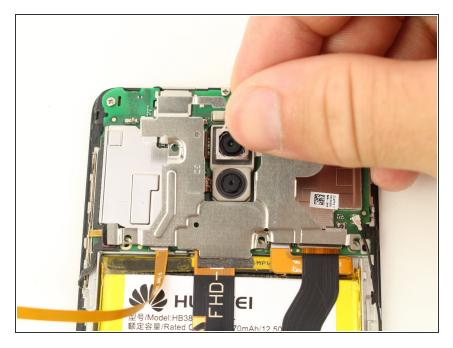
Remove the motherboard cover from the device using a spudger or your fingers.
