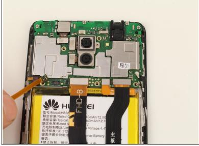
Disconnect the fingerprint scanner cable attached to the motherboard using a spudger or your finger.
