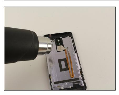
Apply heat around the finger print scanner assembly using a heat gun or hair dryer.
