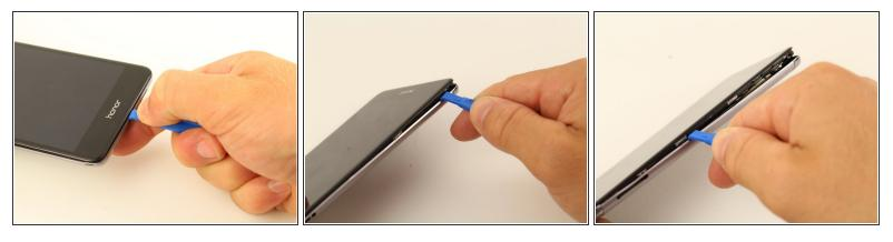
Slide the opening tool or spudger along the bottom of the phone and around the edge.
